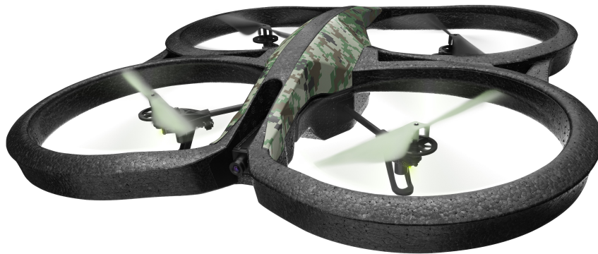
Figure 1: The Parrot AR Drone with the foam indoor shield around the propellers.
